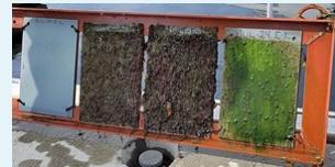
**The Method:** Researchers from the Norwegian University of Science and Technology developed graphene-based polymer nanocomposite coatings that prevent biofouling by physically damaging or deterring organisms on contact, eliminating the need for toxic chemicals.
